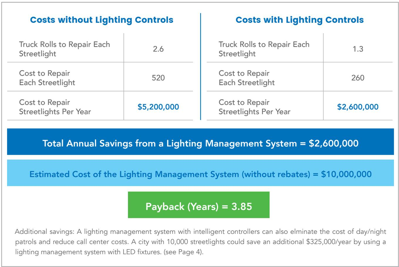
Figure 4: The financial benefit and payback of a lighting management system with intelligent controllers for a city with 10,000 LED streetlights.
