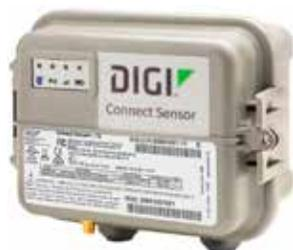
**Digi® ConnectSensor+**- Digi Connect Sensor is a fully integrated, battery powered cellular gateway with I/O for connecting to a wide range of external sensors.
