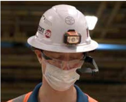
A single onsite Honeywell employee wearing a RealWear device is able to share what they are seeing and engage with offsite expert colleagues through Microsoft Teams in real time. The voice-activated controls enable the wearer to use the various functions — including viewing documents on the high-resolution micro-display, contacting coworkers on Teams, and more — without taking their hands or attention off of complicated machinery or equipment.
