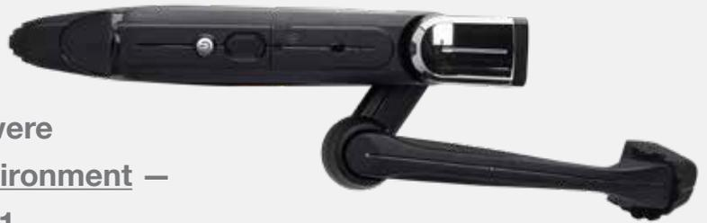
The RealWear HMT-1 is an Android device that has all the capabilities of a tablet but in the form of a headset. The HMT-1 has:
